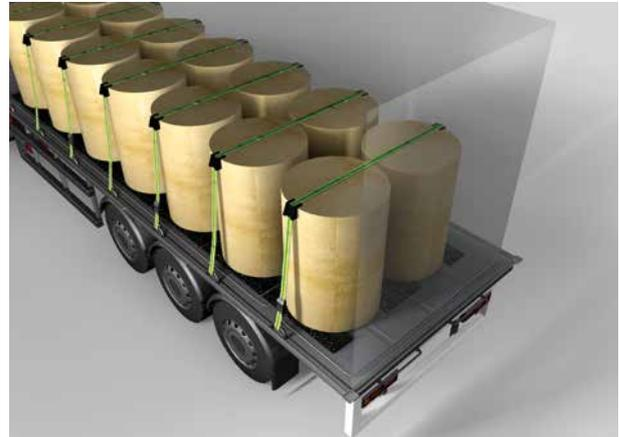
The anti-slip mats must be at least 150 mm wide and 3 mm thick. The length of the mat depends on the diameter of the coils. The anti-slip mats are positioned under the paper coils so that approx. 1 cm of mat can still be seen from the outside.
